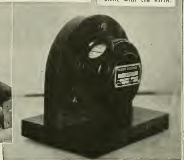
Fig. 4. Dead-beat "Clinometer" which shows angle of aeroplane with the earth.
