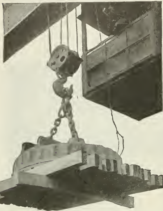
The Crucible Steel Company Have in Use at Their Pittsburgh Plant This Gigantic 62-inch Electro-magnet. It Can Lift 4\frac{1}{2} Tons of Steel Bars and the Trip of a Switch Releases the Entire Load Instantly. This Class of Work Spells "Economy" in Big Letters and Foundries Everywhere Are Rapidly Awakening to the Fact.
