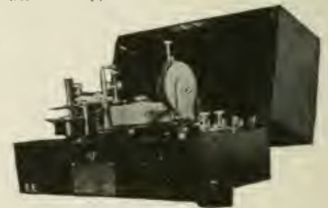
Automatic Code Apparatus Used by U. S. Radio Inspectors in Examining Applicants for Operator's License.
