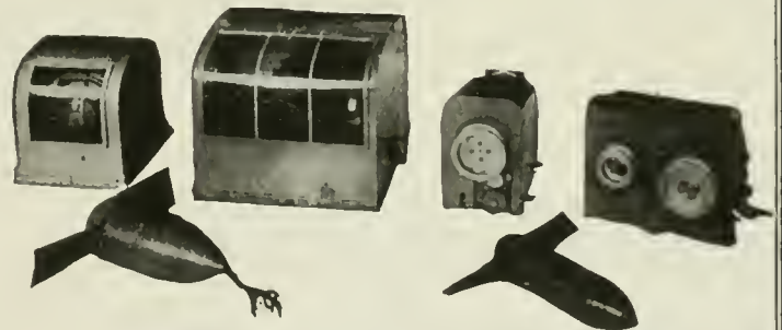
Fig. 5. The "Sperry Automatic Pilot" which, by means of electric driven gyroscopes, serves to control and maintain an aeroplane in any desired position; the pilot may drop bombs, etc.
