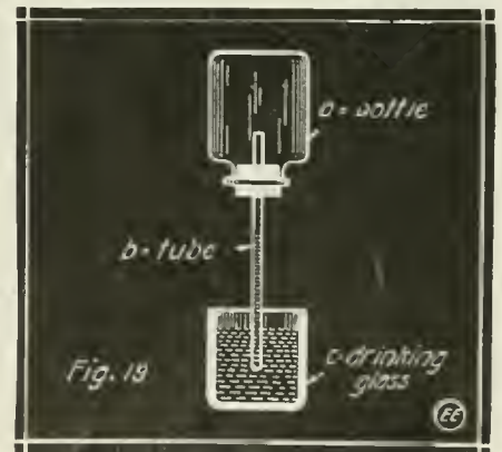
A Simple Air Thermometer—Utilizes the Expansion of Air on Heating to Vary the Height of a Water Column.
